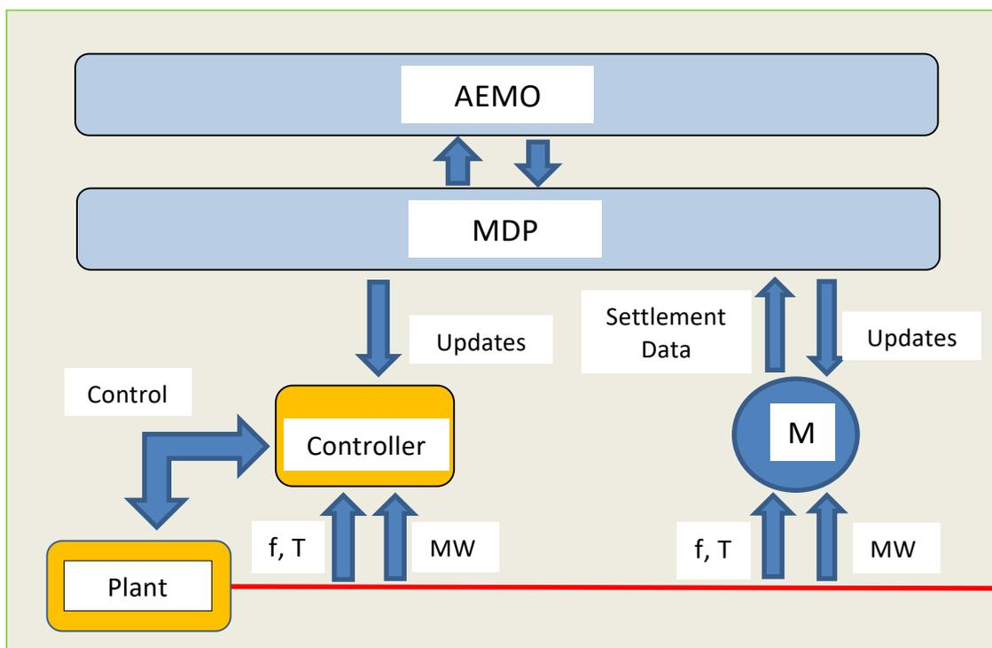
Note that the data going to and from AEMO and the MDP are not required in real time. The strictly real time activity including measurement and control is all handled locally. In this way, very fast responses including inertia can be properly handled.
