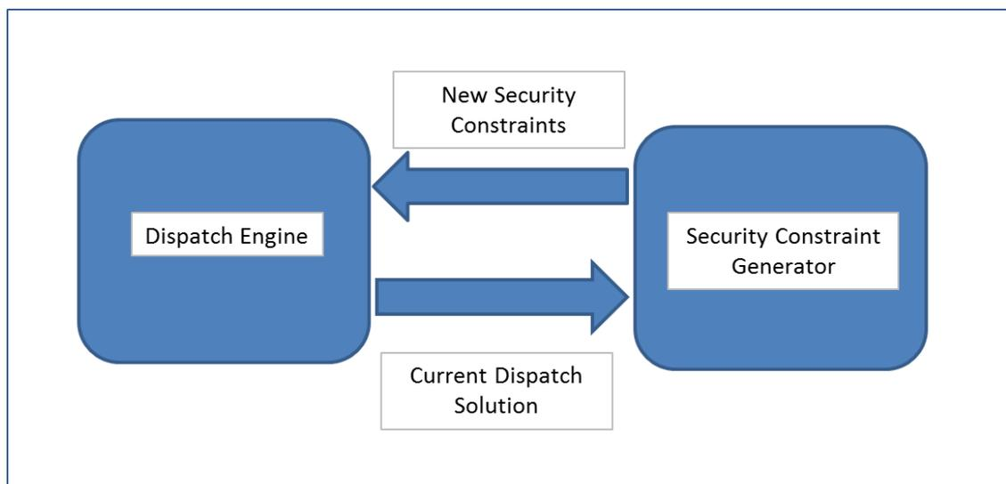
This system does not actually require a network model in the dispatch engine; the security constraint generator has its own network model and can develop constraints in the generic constraint format if required. Constraints generated can take account of dynamic real time data or estimates of the state of equipment (e.g. Its temperature) either directly measured or estimated using a technique such as Kalman filtering.
