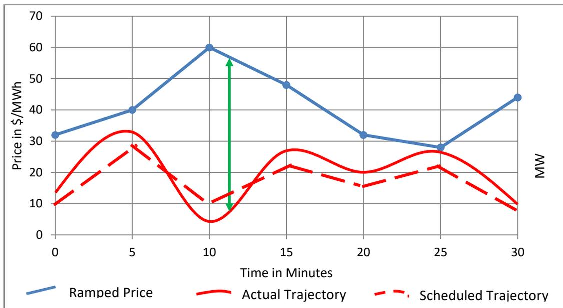
We can carry out the core calculations in real time (either using SCADA or within a specially programmed revenue meter) by accumulating certain measured values for each 5 minutes for later settlement using 5-minute dispatch price data.
